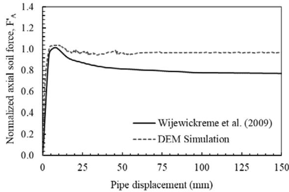
Figure 3. Comparison between calculated and measured pullout response of the pipe
