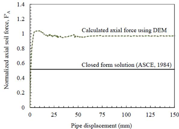
Figure 4. Normalized soil load in the axial direction versus pipe displacement
