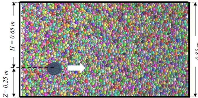
Figure 5. The coupled FE-DE model showing the loaded pipe
