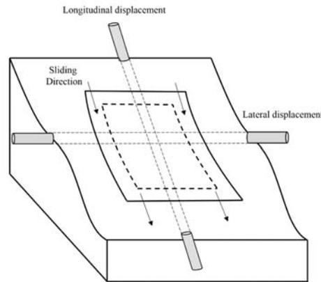
Figure 1. Soil load on pipeline passing through an area subject to landslides
