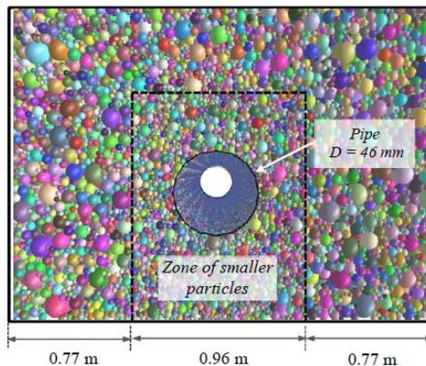
Figure 2. Particle distribution in the close vicinity of the pipe
