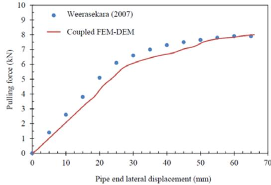
Figure 6. Comparison between the measured and calculated responses of the pipe
